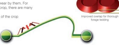
The hay is fully turned over and well aerated thanks to the steep pitch angle for improved drying
