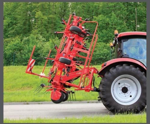
With the GF 8712 and 10812 tedders considerable working width, the smalldiameter rotors limit rear overhang so that it can be used with lower power tractors. The unique folding design allows for exceptionally low transport height and convenient operation from the tractor seat.
