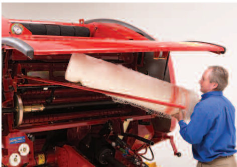
One non-active roll of net wrap can be stored in the front of the baler above the active roll.
