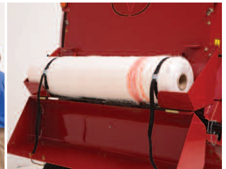
A second non-active roll of net wrap can be stored at the back of the baler.
