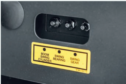
Centralized grease points
