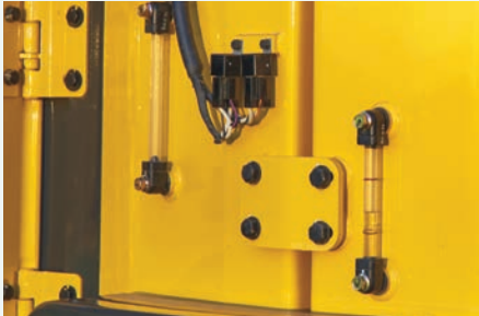
Sight glass allows hydraulic oil level to be checked quickly and with no need to lift the engine hood
